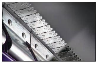
top cover of a belt is greater than 3/16", skiving is always recommended. Skiving does not affect the strength of the belt or the splice because only the top cover is removed, which does not affect the carcass. Deeper penetration of the fastener teeth into the belt carcass can also reduce return idler noise, minimize wear on idler bearings, and eliminate impact with skirting material.
