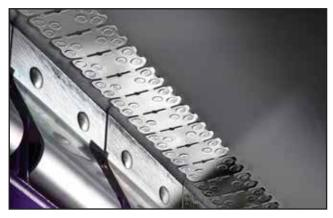
top cover of a belt is greater than 3/16", skiving is always recommended. Skiving does not affect the strength of the belt or the splice because only the top cover is removed, which does not affect the carcass. Deeper penetration of the fastener teeth into the belt carcass can also reduce return idler noise, minimize wear on idler bearings, and eliminate impact with skirting material.
