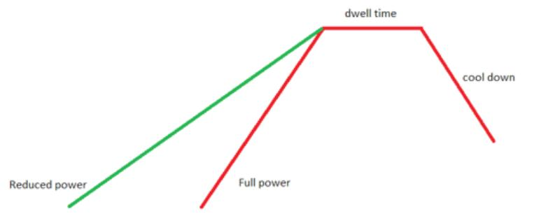
Depending on power used, the press might operate in 'full power' mode, which will have a quicker warm up time, or in the 'reduced power' mode. 'Reduced power' mode will take slightly longer to reach the desired dwell temperature. Actual dwell time and cool down will take the same amount of time in either power mode.
