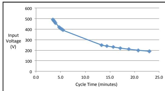
In this instance, the likely culprit is the difference between the 480V and 230V power source, but there are actually a number of factors that should be considered. Here are a few things to think about when voltage variances could be a factor in the length of time to complete a splice:
