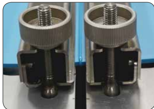
Welded splice prior to skiving bead
